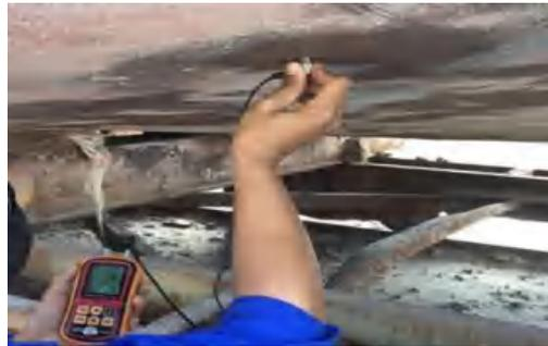
Gambar 3 *Ultrasonic test*
