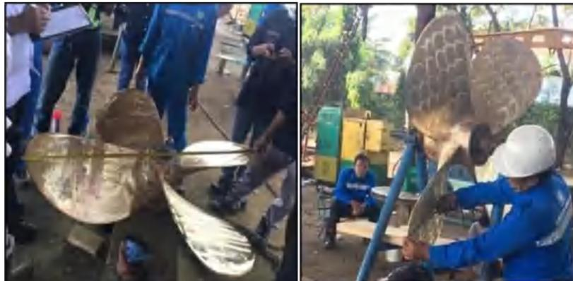
Gambar 2.10 Balancing Propeller
