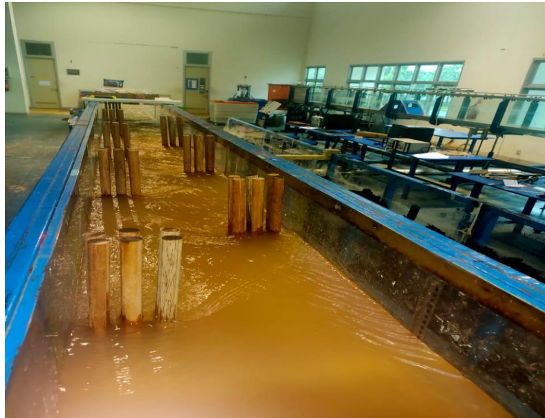
Gambar 32. Pengaliran model krib permeable
