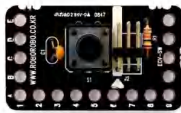
Gambar 5 Contact switch Board
