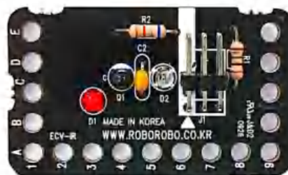
Gambar 6 Infrared Sensor Board
