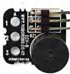
Gambar 4 Buzzer board RoboKit
