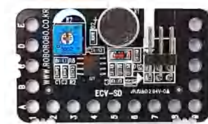
Gambar 7 Sound sensor board RoboKit
