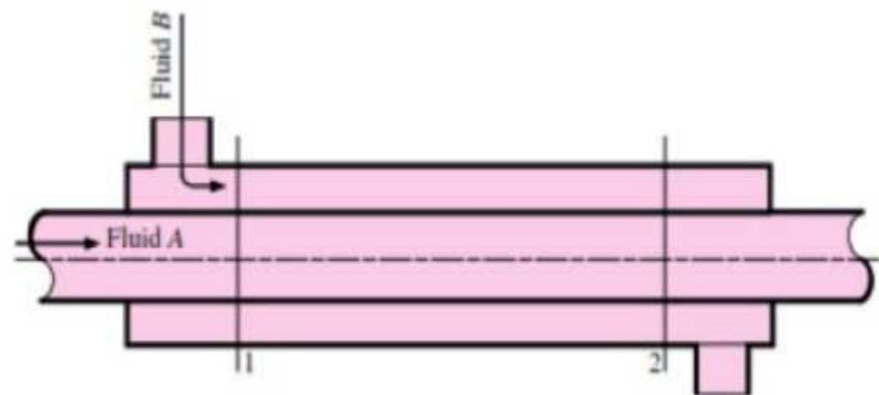
Gambar 6 *Heat Exchanger Tipe Shell and Tube* Aliran Searah
