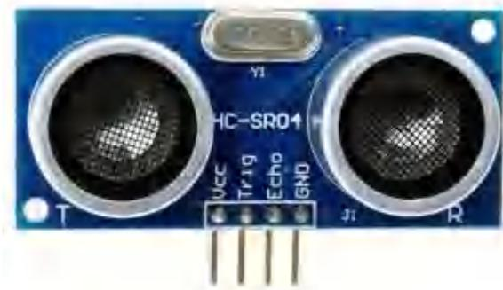
Gambar 11. Sensor Ultrasonik
