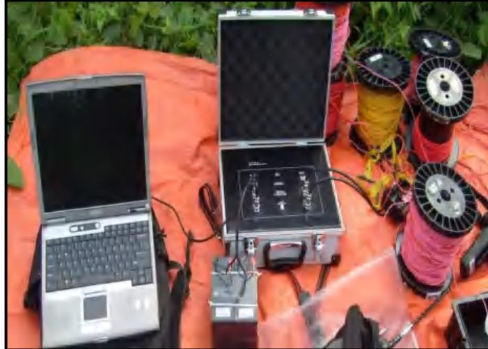
**Gambar 3** Alat Resistivitas S-Field 16 Elektroda *Automatic Multichannel*
