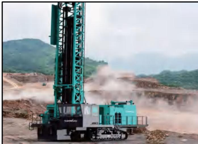
**Gambar 11** *Rotary Air Blasting Rig*
