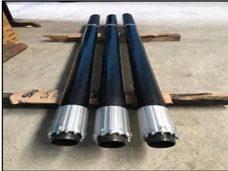
**Gambar 23** Corel Barrel
