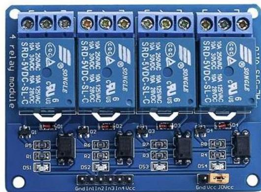
**Gambar 2.5 Relay 4 Channel**
