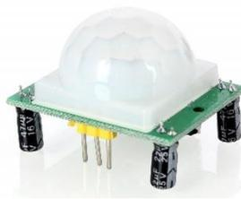
Gambar 2.5 Sensor PIR (*Passive Infrared Received*)
