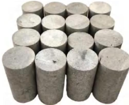
Gambar 2. Beton Silinder
