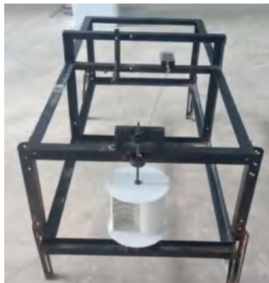
Figure 2. Set up the rotor and instrument model on the frame
