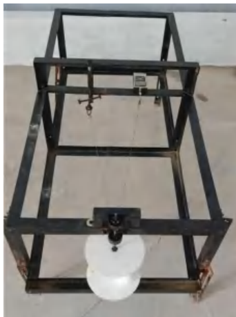
Fig. 3. Set up of the experimental model and instruments on the frame
