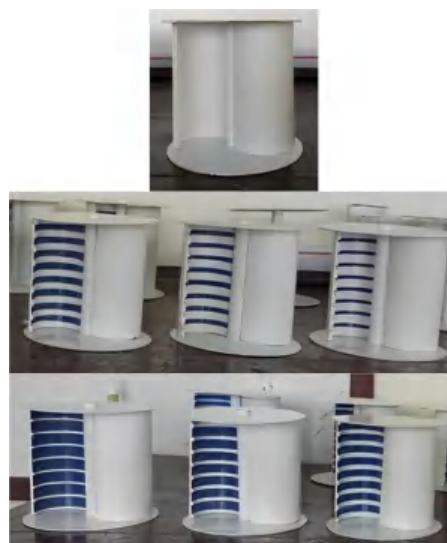
Fig. 2. Eight-grooved blade – 0 mm to 17.5 mm wide
