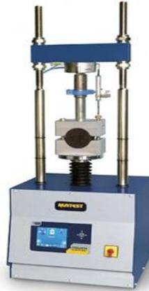
**Gambar 15.** Marshall test set
