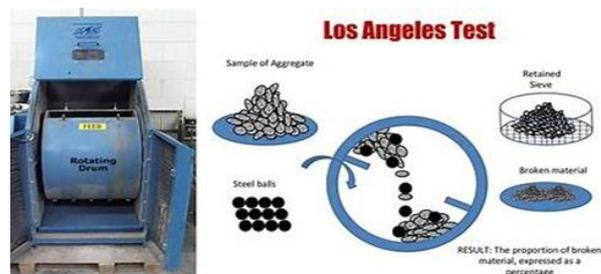
**Gambar 8.** *Los Angeles Abrasion Test*
