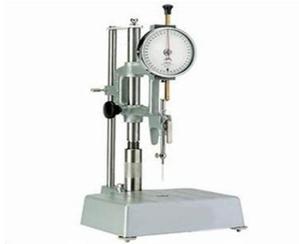
**Gambar 12.** *Hand-operated laboratory penetration test set*
