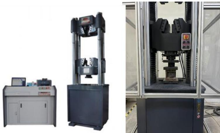
**Gambar 16.** Alat Uji Tekan (*Compressive Test*)
