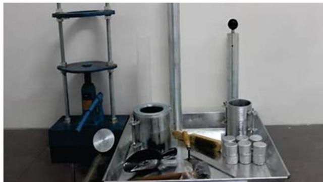
**Gambar 14.** *Compaction test set*
