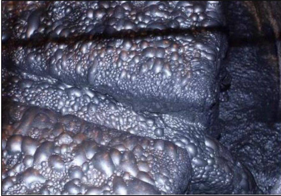
Gambar 6 Air bubbles at the top of a rougher flotation cell.
