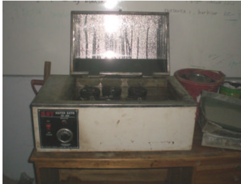
Gambar D13. Alat Perendaman ( Water Bath )
