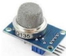
Gambar 3 Sensor Gas  $\text{CO}_2$  (MQ-135)
