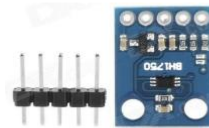
Gambar 9 Sensor BH1750 (Pamungkas dkk, 2015)
