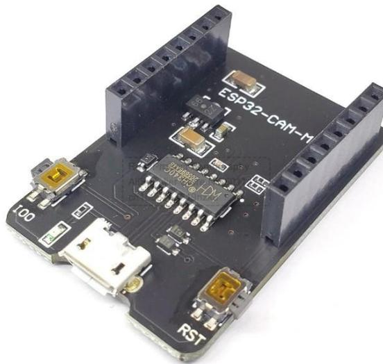
Gambar 2.13 ESP32-CAM CH340 *Development Board*
