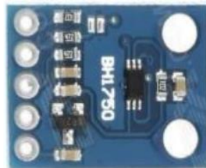
Gambar 3. Sensor Intensitas Cahaya BH1750 [18]
