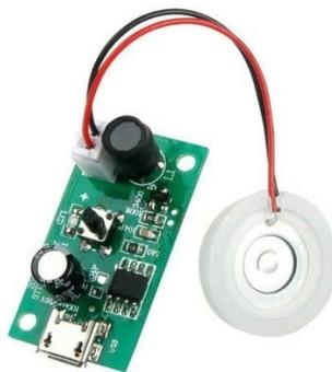
Gambar 8. Module Ultrasonik *Mist Maker*
