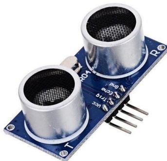
Gambar 3. Sensor ultrasonik HC-SR04
