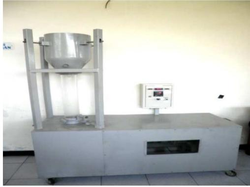
Gambar 7. Alat Pengering Tipe *Fluidized Bed Dryer*.
