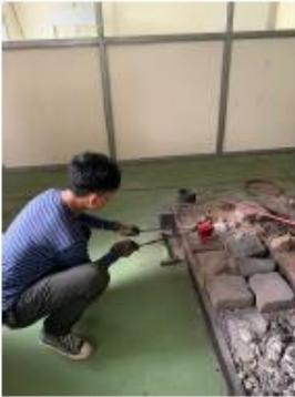
A person wearing a blue long-sleeved shirt and dark pants is crouching on a green floor. They are using a long-handled tool to interact with a furnace or a large container filled with molten material. The furnace is made of brick and has a metal frame. | Dikeluarkannya cetakan dari dalam <i>furnace</i> .            |
