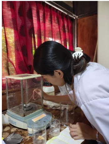
Penimbangan bahan larutan larutan standar
