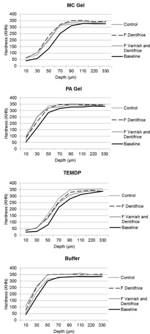
**Figure 4.** Hardness profile (lesion and final) for each type of lesion and remineralising protocol. Footnote: \*Two-way repeated measures ANOVA followed by Bonferroni test ( $p < 0.0001$  for lesion,  $p < 0.0001$  for treatment,  $p < 0.05$  for interaction between factors at 10, 90, 110, and 330  $\mu\text{m}$  and  $p > 0.05$  at 30, 50, 70, and 220  $\mu\text{m}$ )
