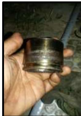
Gambar 2.5. *Piston Caliper*
