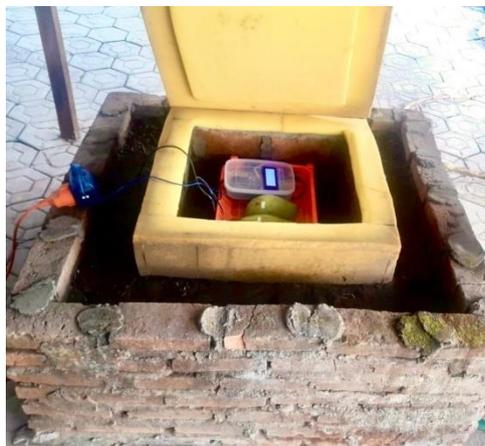
Gambar 2. *Zero Energy Cool Chamber* (ZECC)
