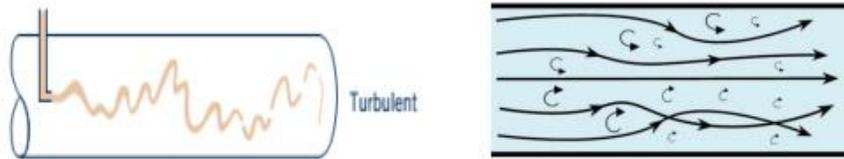
**Gambar 7.** Aliran Turbulen
