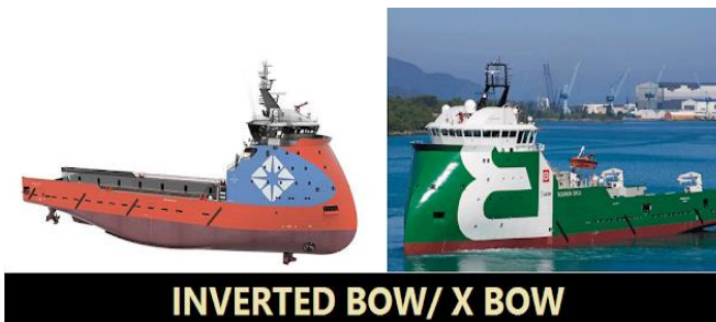
Gambar 10. Haluan Kapal Inverted Bow / X Bow
