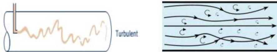
**Gambar 13.** Aliran Turbulen
