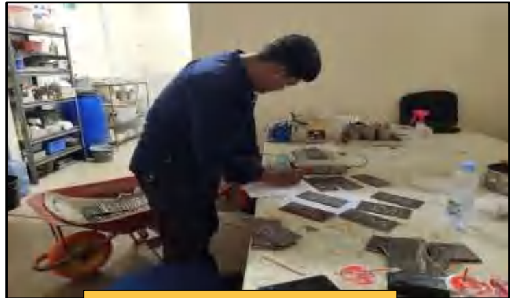
Menimbang berat awal benda uji (ASTM G1)
