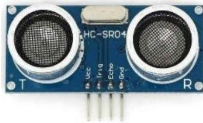
**Gambar 2.4** Sensor ultrasonik HCSR-04 [15]
