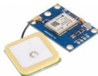
**Gambar 2.4** Modul GPS uBlox NEO-6MV [20]
