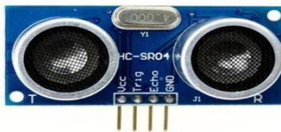
**Gambar 2.2** Sensor ultrasonik HC-SR04 [16]
