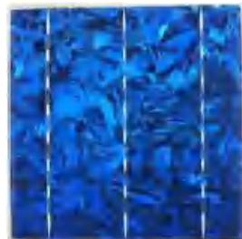
**Gambar 2** Panel surya polycrystalline (Kencana et al., 2018)
