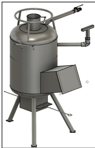
Gambar 7. Tungku biomassa injeksi uap over fire
