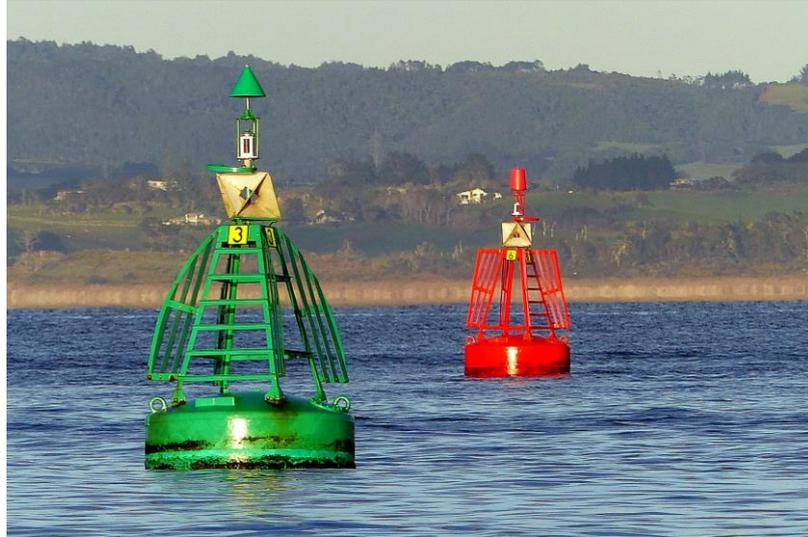
Gambar 3. *Buoy Lateral*
