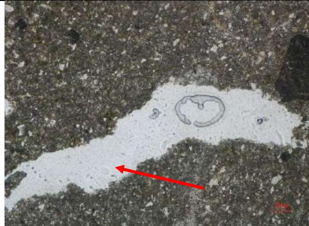
A micrograph showing a large, irregularly shaped, light-colored area representing dissolution (channel porosity) within a dark, granular matrix. A red arrow points to the boundary of this porous area.                                                                       |
