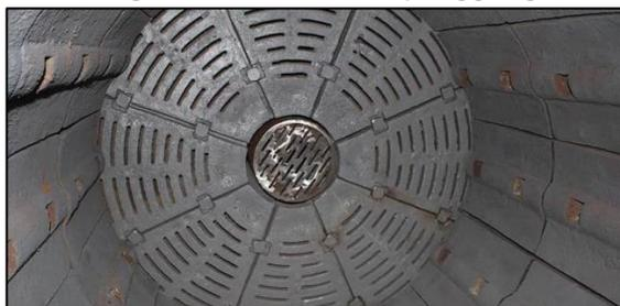
**Gambar 12.** *Liner ball mill*
