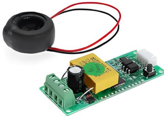
Gambar 10. Sensor PZEM-004T (Ibrahim, Ridyandhika Riza , Bekti Yulianti, 2022)
