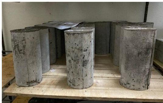
Lampiran 4 Proses moist curing beton geopolymer
