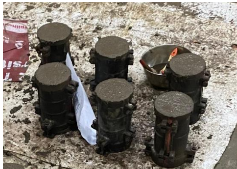
Lampiran 3 Pengecoran beton geopolymer
