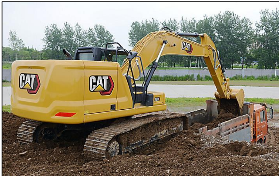
Gambar 3. Backhoe Cat 320 NG (Caterpillar, 2023)
