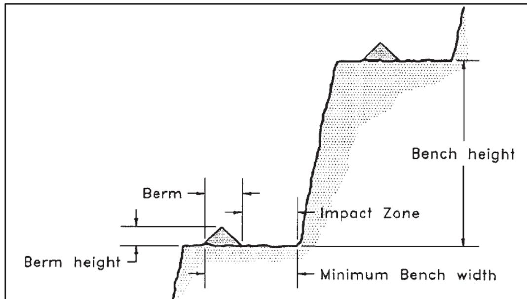
Figure 6 Catch bench geometry (Hustrulid et al., 2013)
