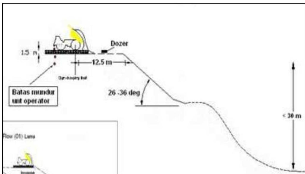
Figure 11 Semi induced flow disposal (PT Vale Indonesia Tbk, 2018)
