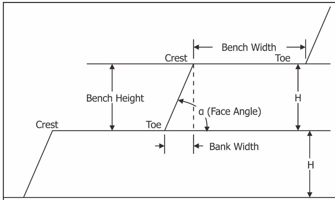
Figure 4 Parts of a bench geometry (Hustrulid et al., 2013)
