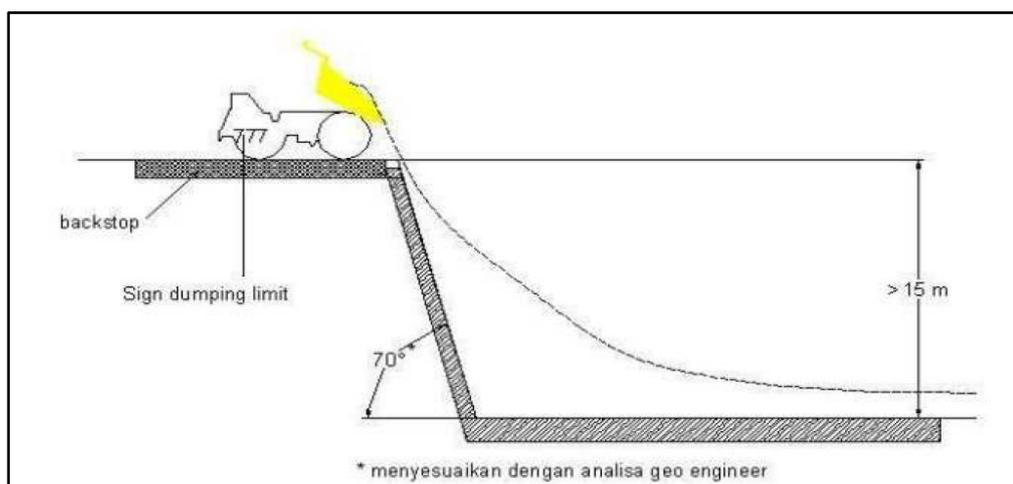
Figure 10 Induced flow disposal design (PT Vale Indonesia Tbk, 2018)
