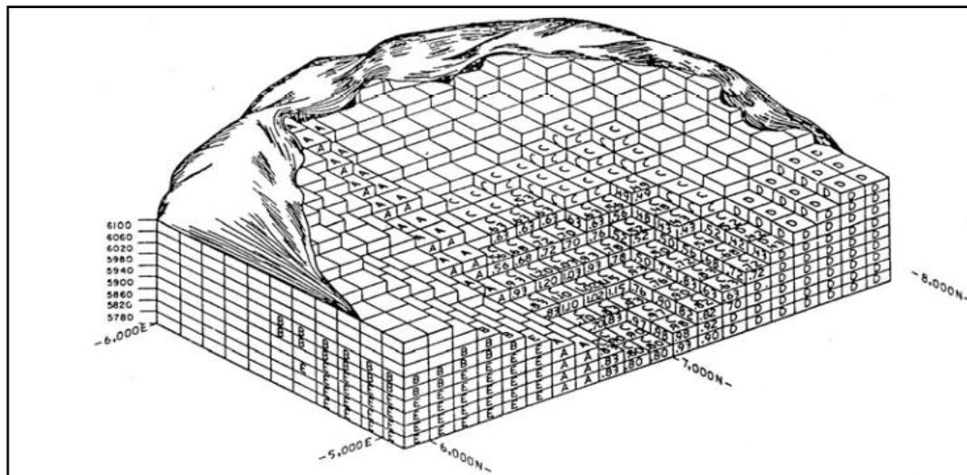
Figure 8 Reserve calculation with block model method (Sinclair and Blackwell, 2002)
