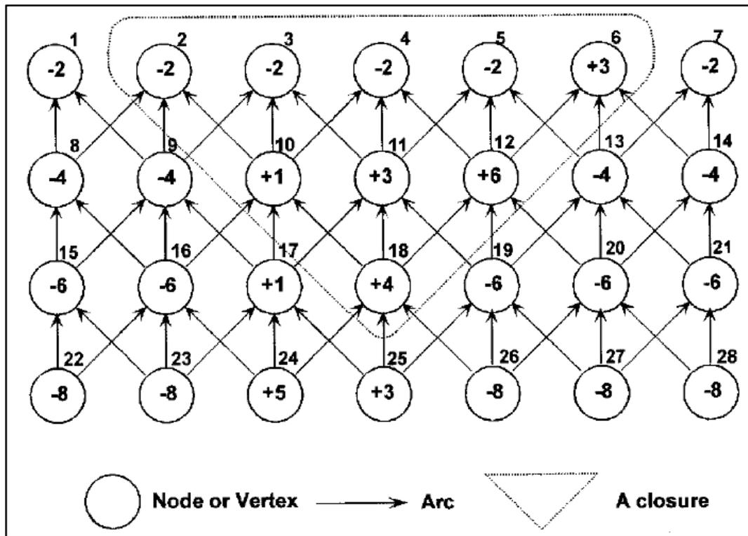
Figure 2 Directed graph representing a vertical section (Khalokakaie et al., 2000)
