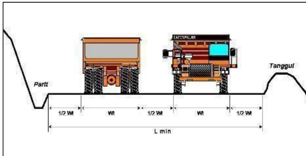
Figure 7 Parts of mine road (Hustrulid et al., 2013)
