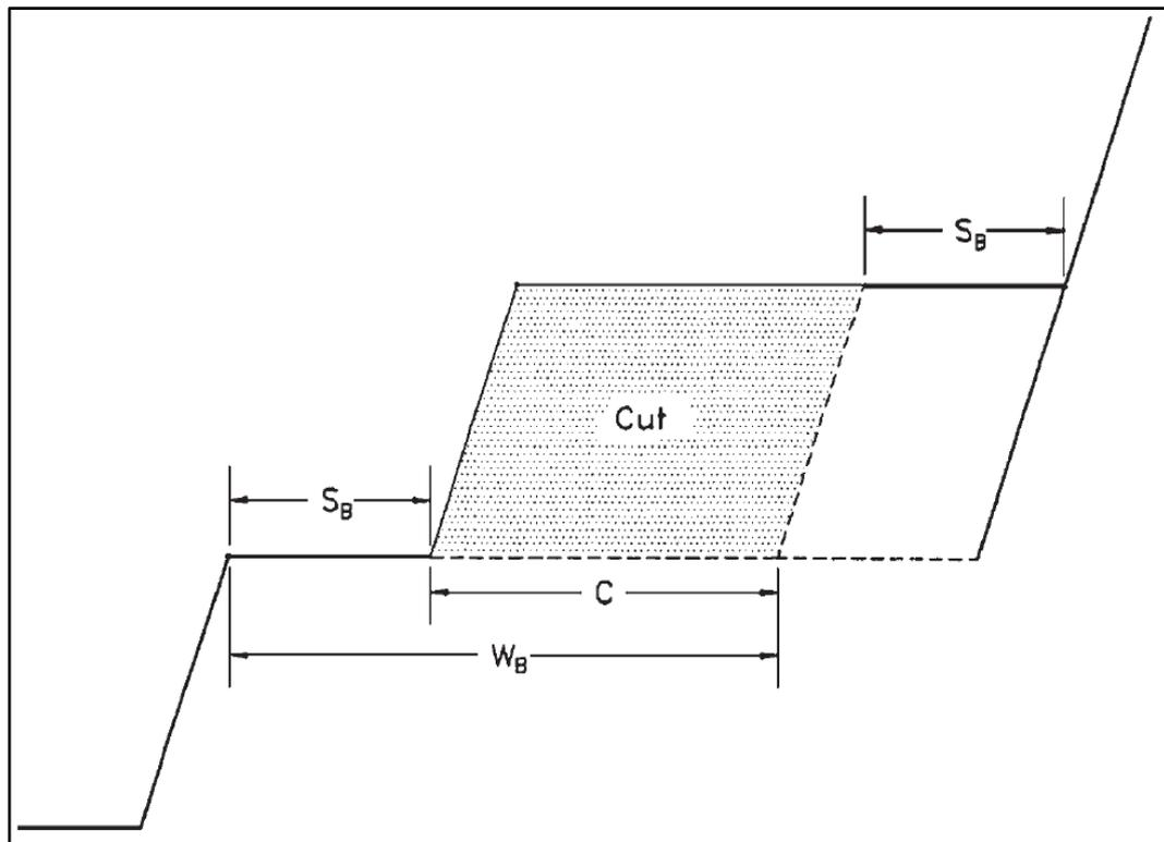
Figure 5 Parts of working bench (Hustrulid et al., 2013)
