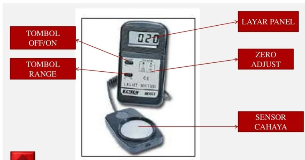
**Gambar 2.3 Bagian-bagian Lux Meter**
