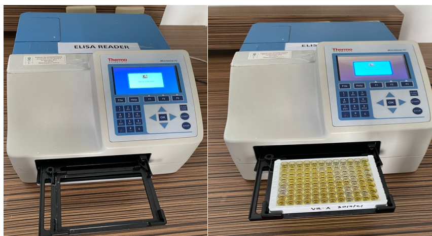
Gambar 2. ELISA Reader. Thermo Scientific™ Multiskan™ FC Microplate Photometer
