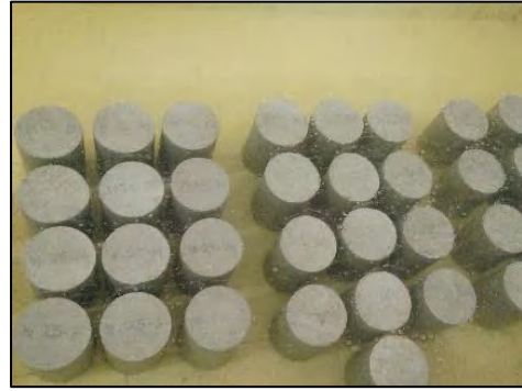
Perawatan benda uji ( Wet curing )
