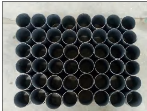
Bekisting Silinder 10 cm x 20
