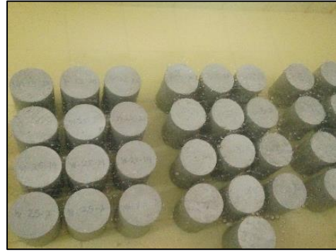
Perawatan benda uji ( Wet curing )
