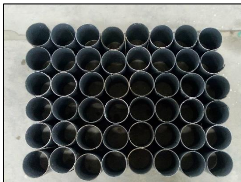
Bekisting Silinder 10 cm x 20
