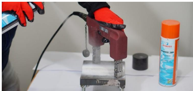
Gambar 14 Magnetic Particle Inspection
