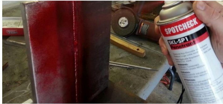
Gambar 15 Dye Penetrant test
