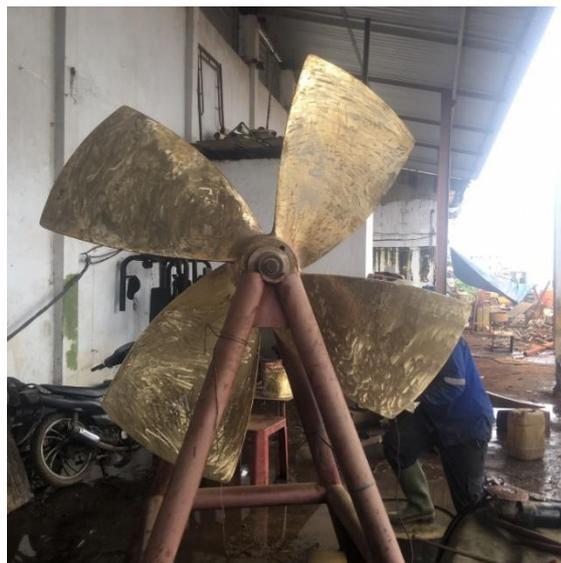
Gambar 5. Proses balancing propeller
