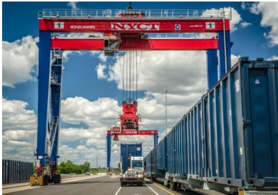
Gambar 2.3 Rubber Tyred Gantry (RTG) Crane
