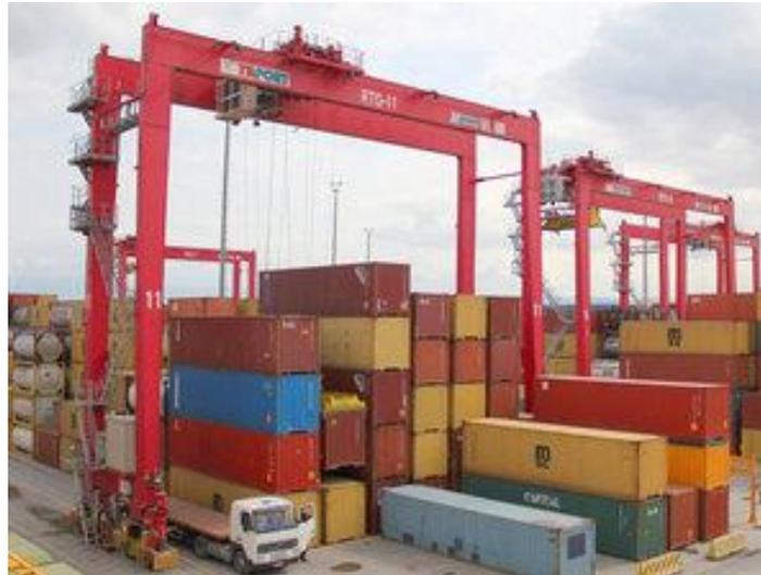
**Gambar 6.** Rubber Tired Gantry (RTG)
