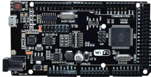
Gambar 2. 3 Arduino Mega 2560 Wifi Built-in – ESP8266
