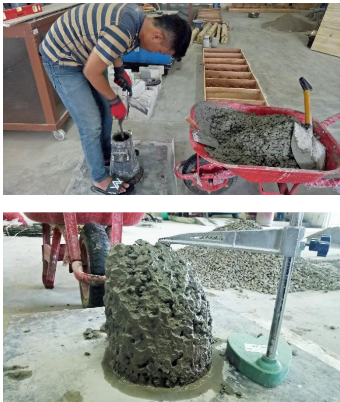
Gambar 4.12 Pengujian Slump Campuran Beton
