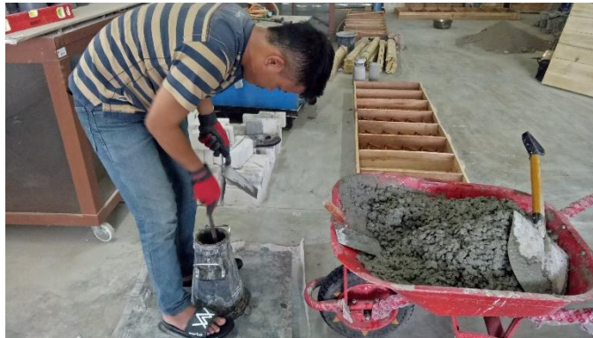
Gambar 6.19 Pengujian Slump Campuran Beton
