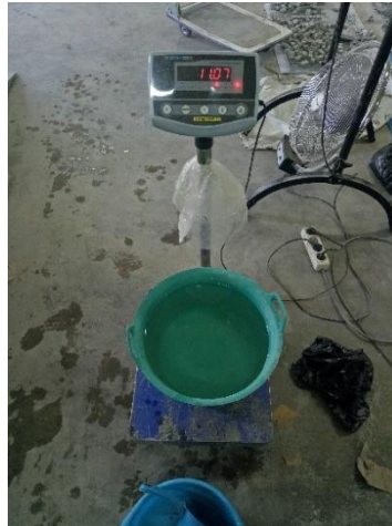
Gambar 6.16 Penimbangan Material Beton
